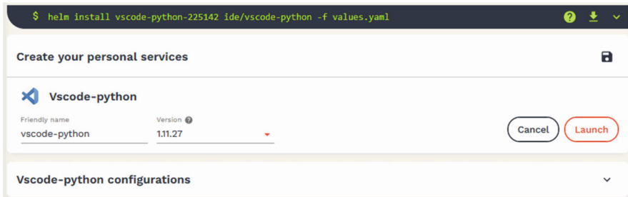
Fig. 8.5 Launching a service through Onyxia’s UI. Note: Services from Onyxia’s catalog can either be used vanilla or configured by the users to tailor them to their specific needs. In order to limit the dependence of users on Onyxia, each action performed by the user on the UI is accompanied by the actual command that is executed on the Kubernetes cluster
